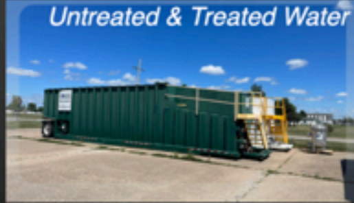
Flotation Mobile Treatment Unit (MTU)
